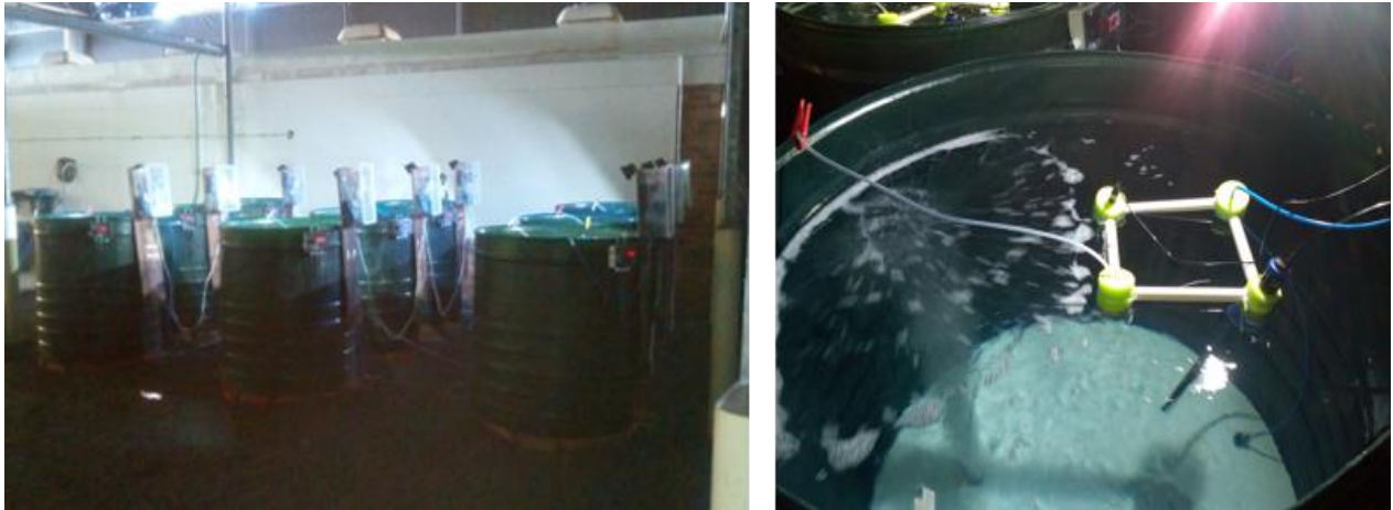
Figure 2. 3: Non-recirculating system used in rearing Argyrosomus japonicus , a) the nine independent experimental tanks and b) the inside of the tank showing the white painted floor.
