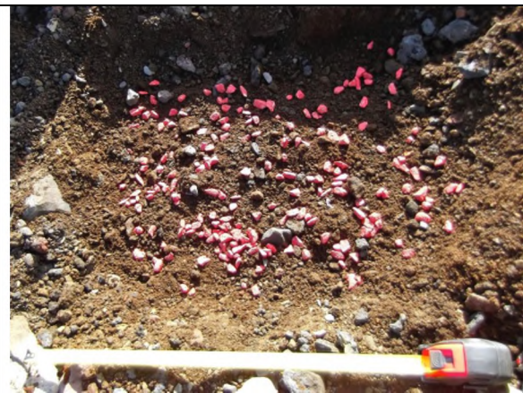
Figure 45: Markers at 10 cm depth. Scale: 50 cm.
