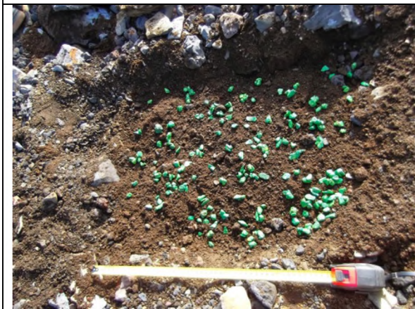
Figure 44: Markers at 5 cm depth. Scale: 50 cm.
