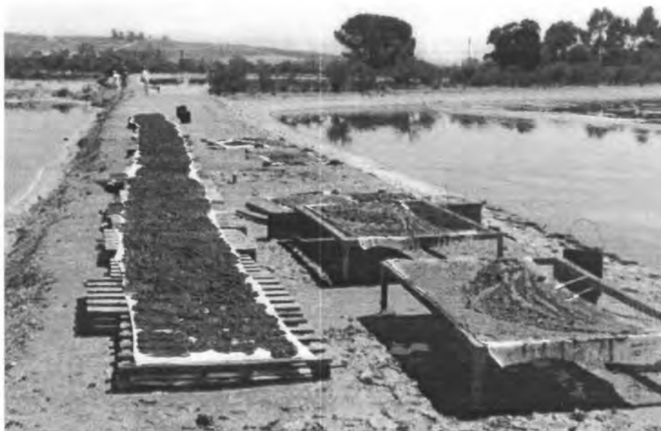
Figure 6.4.2. The sun drying beds used at Mossop Western Leathers, Wellington.
