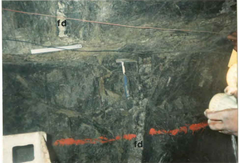
Fig.3.10 Unki stope. Footwall Shear showing sinistral displacement (horizontally) of felsic dykes (fd). [2 level drive north, looking east].
