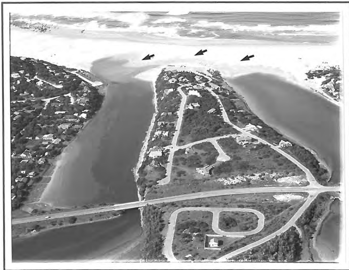
Plate 2.1 The mouth regions of the East and West Kleinemonde estuaries showing the accumulation of sand (indicated by arrows) which moves mostly in an north-easterly direction (Photograph: A. K. Whitfield, May 1993).
