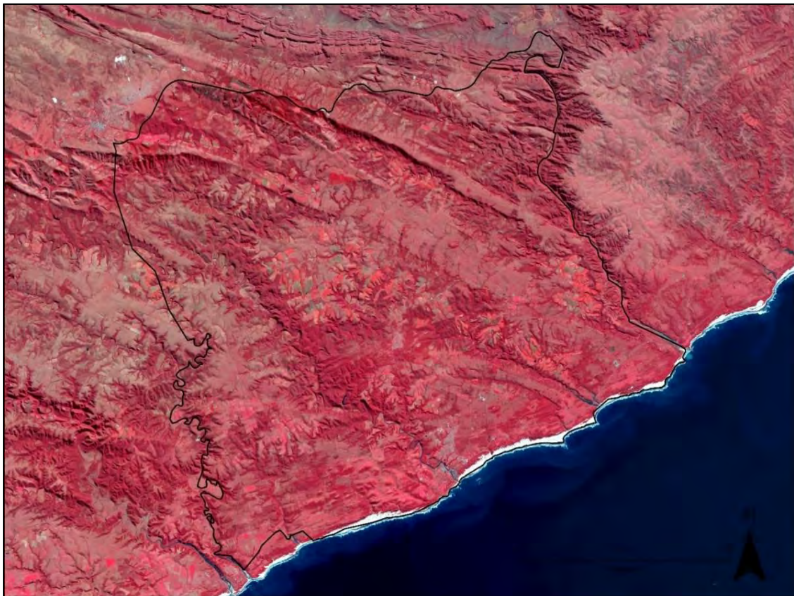
Figure 35: Landsat 8 false colour image (bands 7, 6, 4) of the study area (Source: USGS Earth Explorer https://earthexplorer.usgs.gov/ ) [Accessed 02-07-2023].
