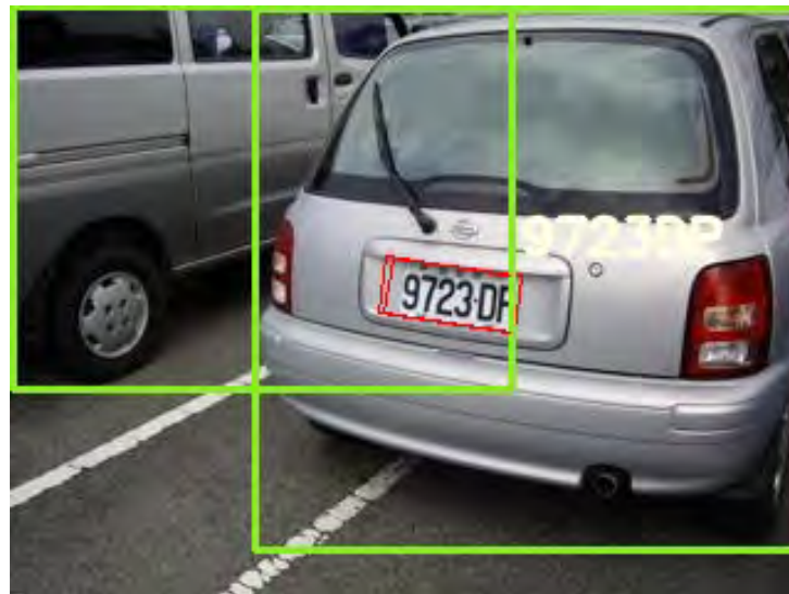
Figure 5.43: The intersection of the two-vehicle bounding boxes includes the same licence plate, resulting in a duplicate detection.
