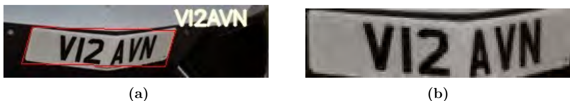
Figure 5.20: The IWPOD-NET cuts off portions of the licence plate to accommodate a quadrilateral shape. While the YOLOv7 model can still read the licence plate, the characters in the image are not horizontally aligned, which can cause incorrect detections in less trivial scenarios.
