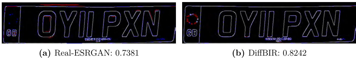
Figure 5.22: The DiffBIR model achieves near-perfect restoration, showing only a few red lines where the model tried to reconstruct fine details.
