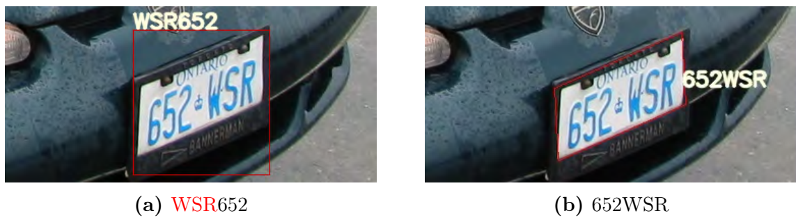
Figure 5.17: Capturing a licence plate with a bounding box makes it difficult to place characters in the correct order.
