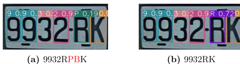
Figure 5.35: Without class-agnostic NMS, predicted strings from the model are longer and inaccurate as every detected character is included in the string, including overlapping predictions.
