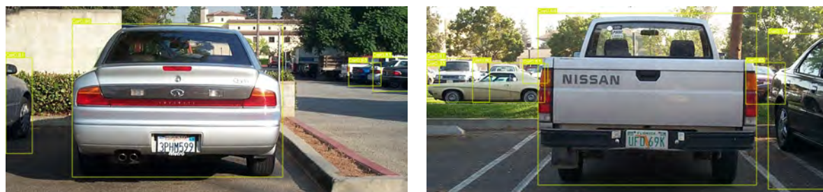
(a) The red vehicle, which is the furthest away from the camera, is undetected. (b) A particularly crowded scene with many occluded vehicles.
