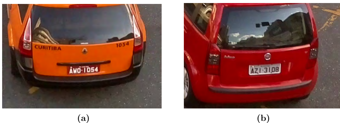
Figure 2.8: Characters on Brazilian licence plates such as [0, O] [1, I] are identical (De Oliveira et al. , 2021).
