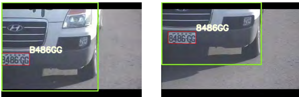
(a) The first character of the licence plate is truncated because it is out of the camera's field of view. (b) When the vehicle licence plate is in full view, there is no issue correctly classifying the character.
