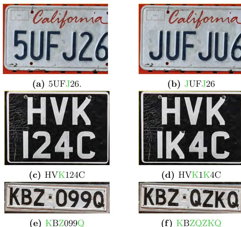
Figure 4.4: Using ground truth bounding box labels, underrepresented character classes were increased by imposing them over classes with enough samples throughout the dataset.
