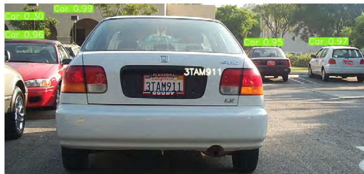
Figure 5.10: The IWPOD-NET model could locate all visible licence plates in the image.
