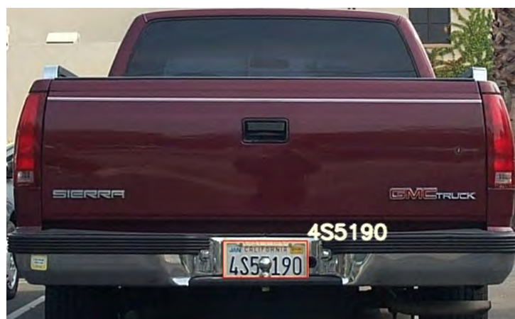
Figure 5.38: The fourth character on the licence plate is blocked by the tow bar on the vehicle, resulting in a missed detection.
