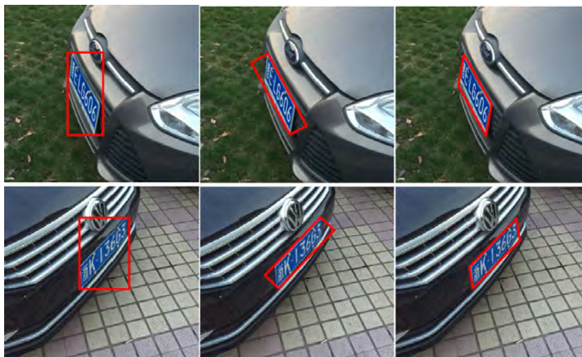
Figure 2.7: From left to right, variations of bounding shapes include a standard bounding box, an oriented bounding box and a bounding parallelogram. The bounding parallelogram is the most effective way to capture the ROI with minimal background noise.
