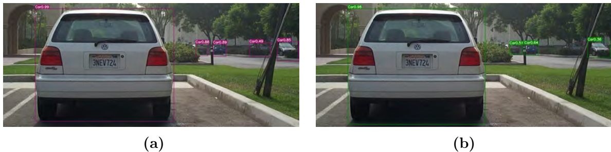
Figure 5.5: The tiny model (5.5b) failed to detect one of the distant vehicles, while the larger model was able to detect it despite it being behind a tree.
