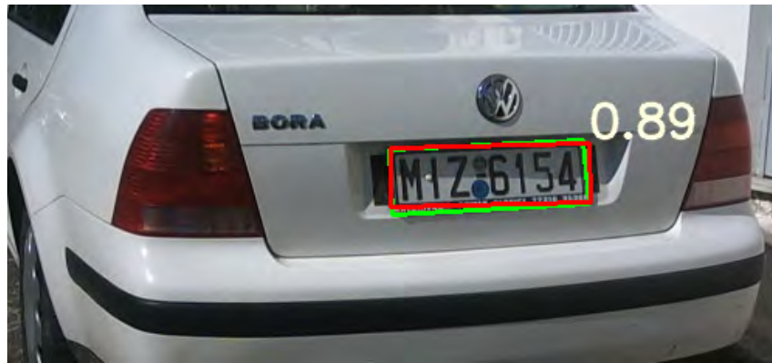
Figure 4.8: IoU is represented by the intersection of the ground truth (green) and prediction (red).
