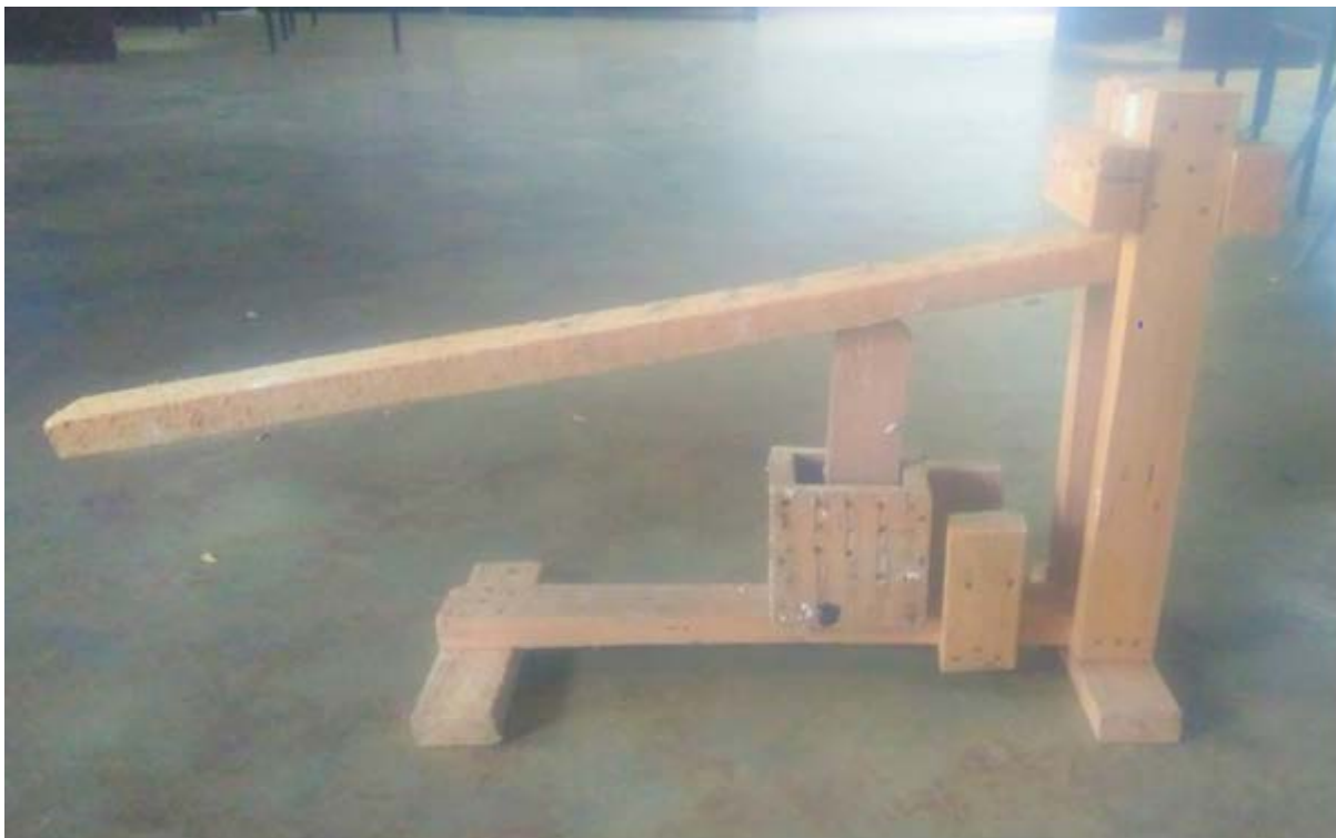
Figure 5.4: Simple briquette machine made from wood
