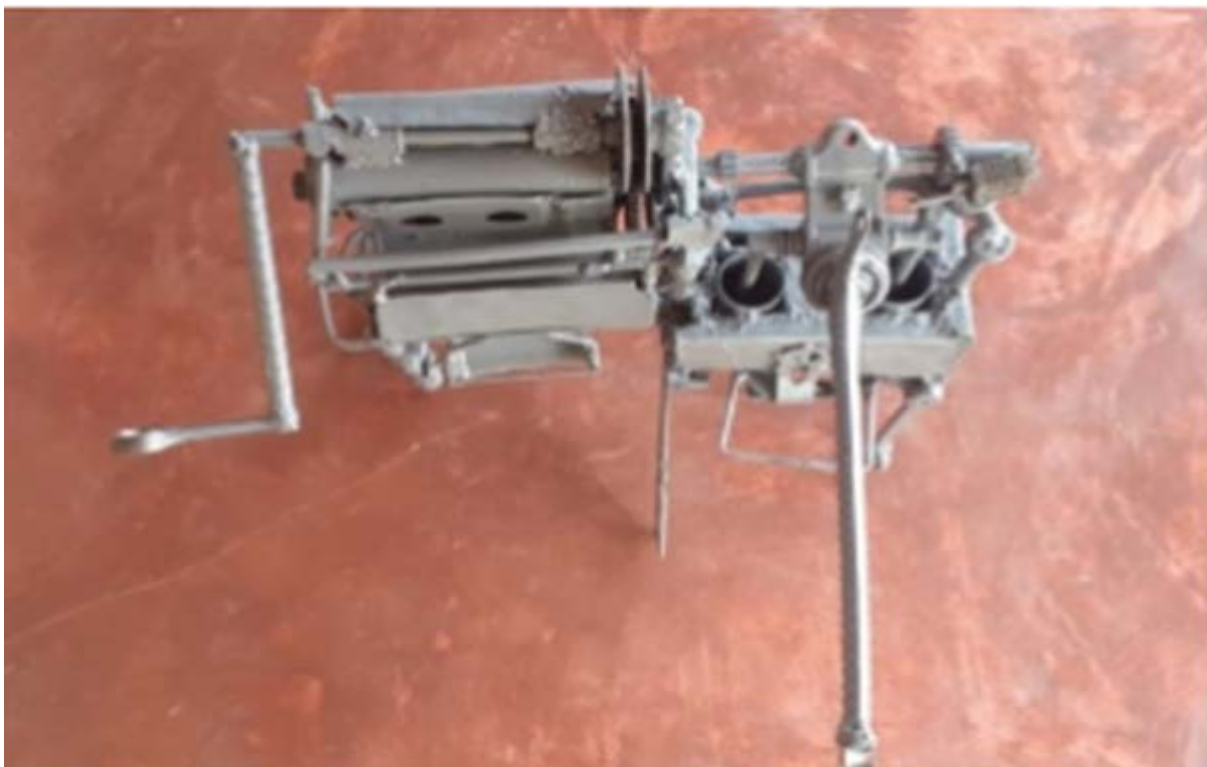
Figure 5.5: Briquette machine made from waste metal
