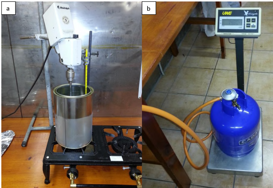
Figure 8a. The pasteurization tin placed on a gas plate that is connected to an LPG cylinder. The overhead stirrer and a thermometer are immersed on the effluent. 8b, the LPG cylinder on a scale used to determine the amount of gas used.
