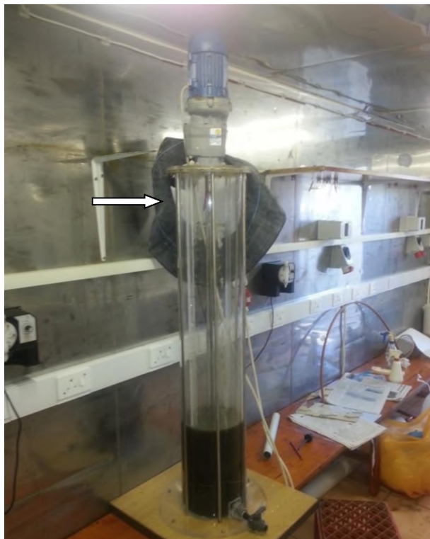
Figure 6. The Perspex digester used for anaerobically digesting pit latrine faecal sludge. An inner tube of a car tyre (white arrow) was attached to the top of the digester collected biogas
