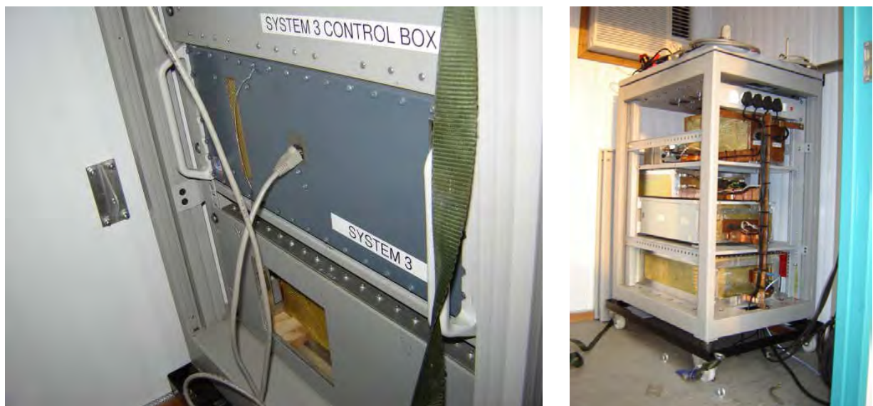
Figure B.2: Top: One of the RFI measurement systems during field measurements at a remote site in the Karoo. Bottom: The measurement equipment installed in the rack of the measurement trailer. The front of the rack (left) is shown with the spectrum analyser, Control PC and Electronics Control Box installed. The Ethernet cable for providing control of the Control PC via the laptop is connected to the front of the Control PC. The back of the rack with copper busbar attached to the rack-mount instruments and the cabling are shown in the image on the right.
