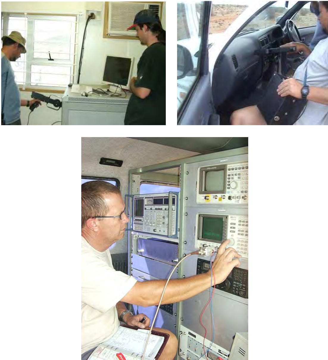
Figure C.1: Photographs of the procedures undertaken to identify RFI sources at the Karoo 3 core site. Top: The handheld directional antenna (Rohde & Schwartz HE200) is used to locate interference in the equipment rack (left) inside the site container and the vehicles on site (right). Bottom: Equipment in the ICASA DF vehicle is used for coarse direction finding of the RFI sources.
