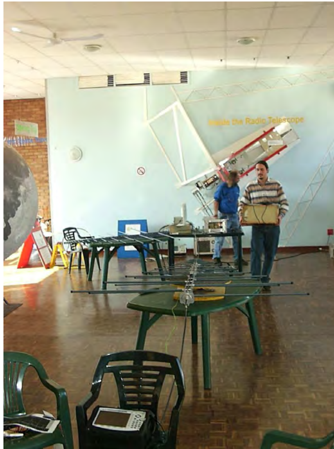
Figure C.3: Photograph taken in the HartRAO Visitors Centre during preliminary validation of the screening on RFI measurement System 2. The Anritsu portable spectrum analyser (on chair in the foreground) is connected to the R & S HL033 antenna which is directed at the RFI measurement system components on the bench.
