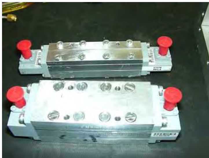
Figure A.4: The 11.5 GHz and 17.5 GHz image rejection high pass filters used in System 1.
