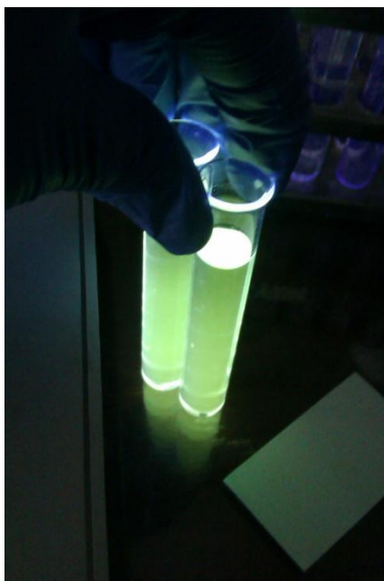
Figure 3.10 Fluorescence of compound 1.64 (roughly 0.1 mg) when irradiated with ultraviolet light (365 nm) This fluorescence was observed for all thiazoles synthesized.
