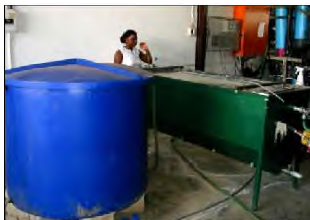
Figure 7.8 A lignocellulose packed sulphide generator (blue tank) providing feed to the floating sulphur biofilm reactor.
