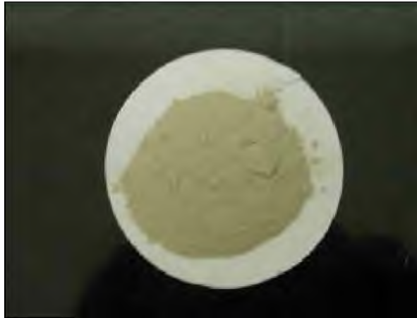
Figure 2.8 Dried floating sulphur biofilm sample from the harvested sediment accumulated at the bottom of the linear flow channel reactor.
