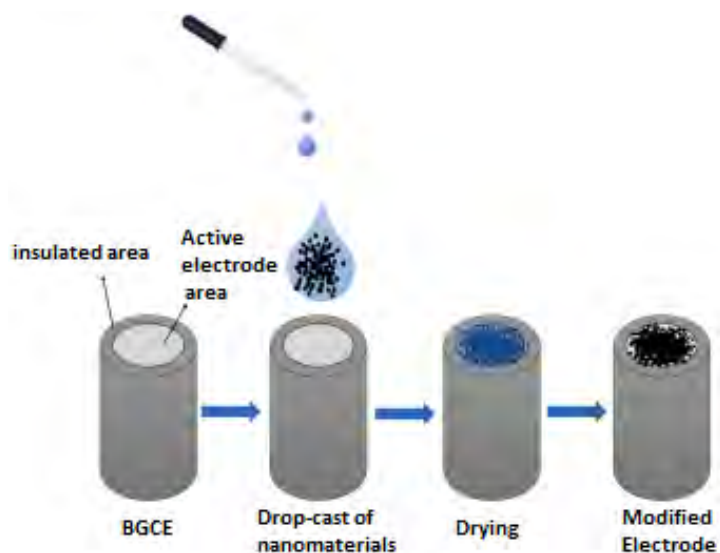
Figure 1.8. A schematic showing the drop-dry method for electrode modification [155]. BGCE = bare glassy carbon electrode
