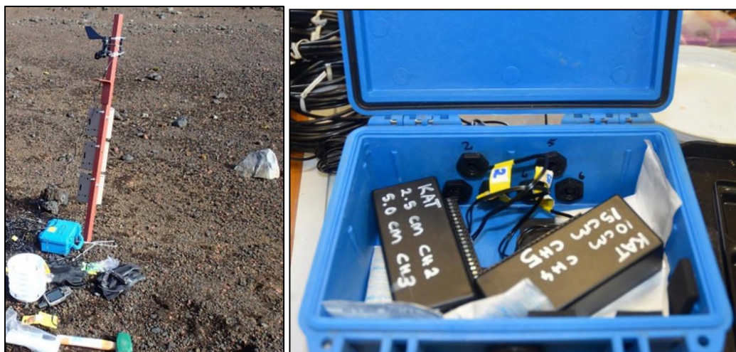
Figure 4.11. Deploying the metal pole Figure 4.12. Weatherproof case with XR-5 loggers (Photo: J. Rosenfels)
