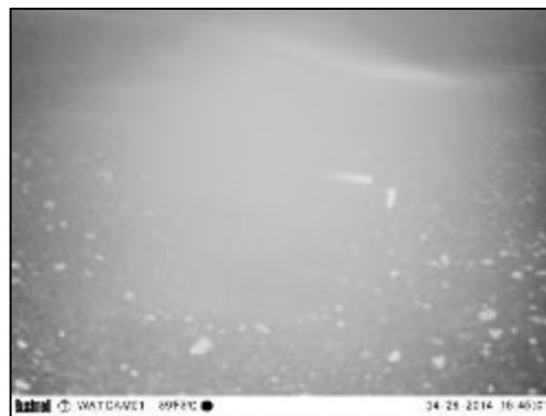
Figure 4.19. Icing up of camera lens by wind and snow
