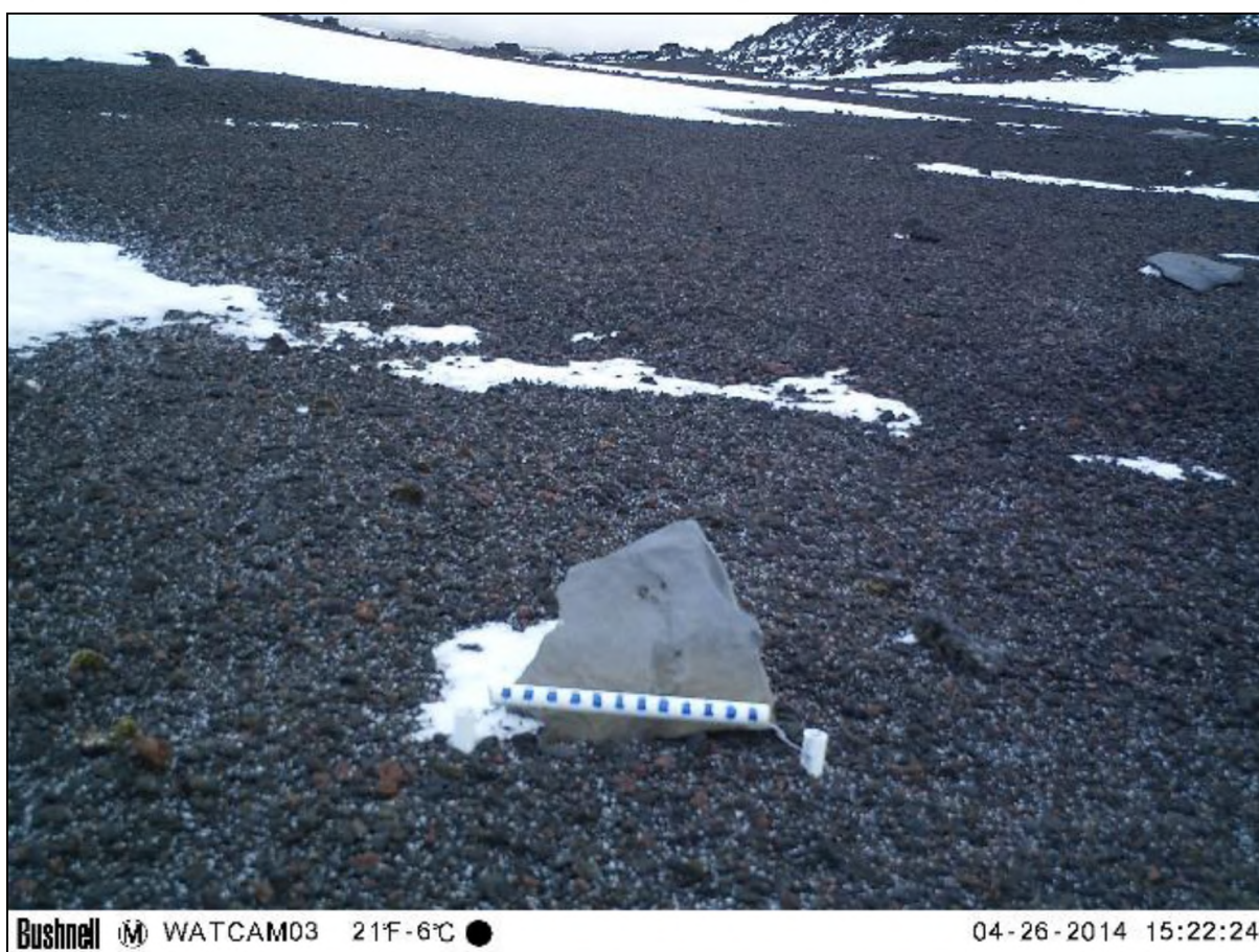
Figure 4.1. Image showing the 25-cm long PVC scale bar used for in scale measurement of clast movement at Site 3
