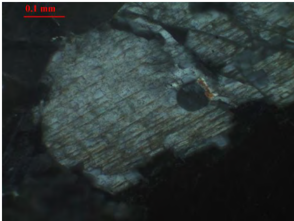
Figure 13b: Photomicrograph taken from slide P3 of plagioclase chadacryst within coarse-grained tabular orthopyroxene with associated clinopyroxene reaction rim.
