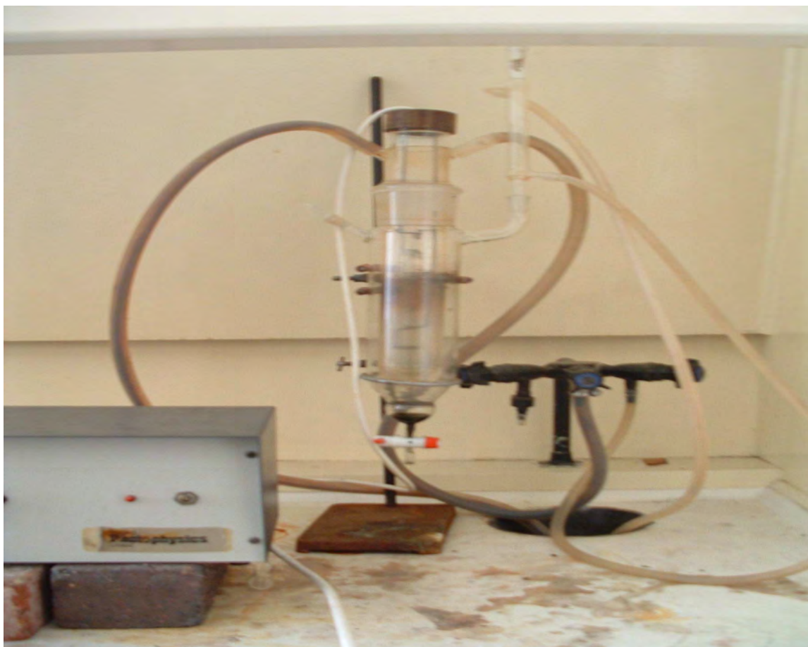
Figure 3.1 The immersion well-photoreactor used to synthesise 3-methoxy-2-formyl pyrrole ( 47 ).
