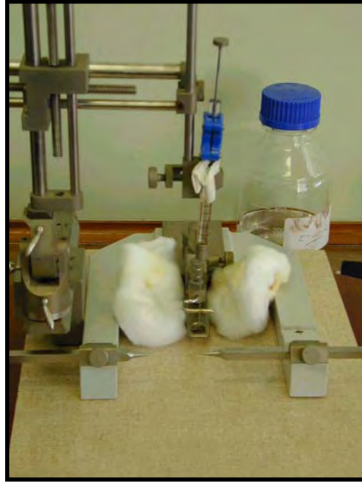
Figure 2.4 A view of the stereotaxic apparatus used for the bilateral intrahippocampal injection of QUIN
