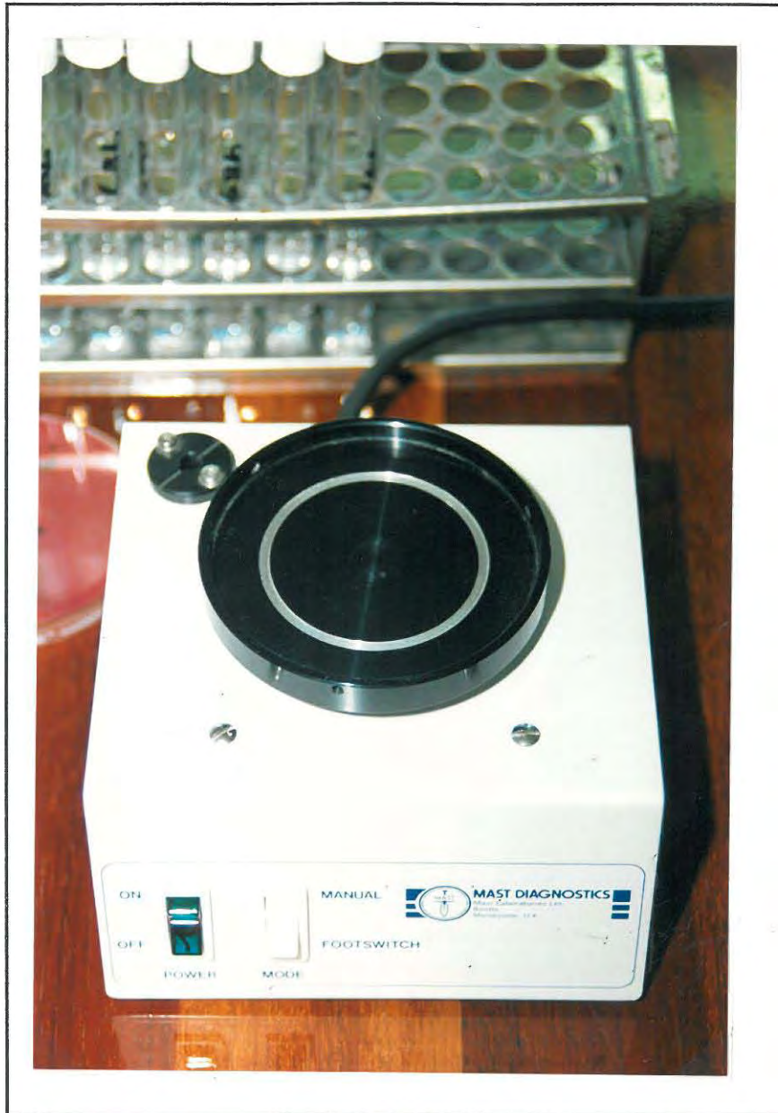
Figure 2.1. The "MAST" rotary plater.
