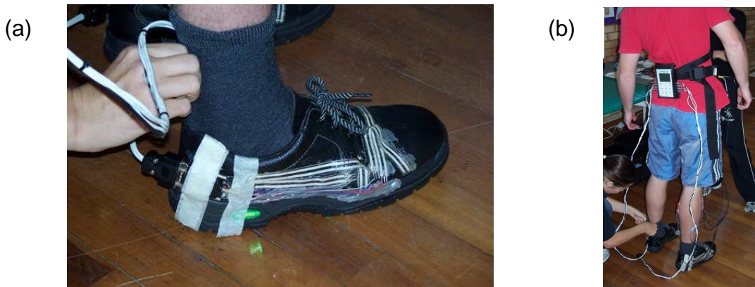
Figure 7: Work boots used in the current study illustrating (a) the built in contact sensors with (b) connection to the DataLOG.
