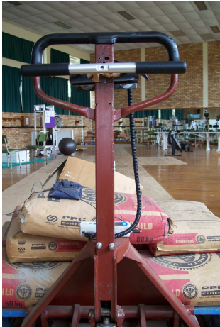
Figure 5: Modified pallet jack handle with Chatillon™ load cell attachment.
