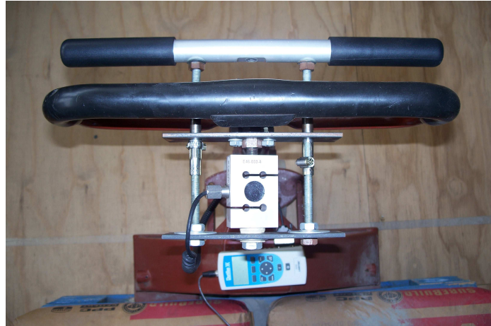
Figure 5: Modified pallet jack handle with Chatillon™ load cell attachment.
