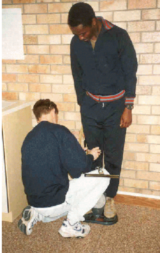
Figure 16: Setup procedure for leg and back strength dynamometry
