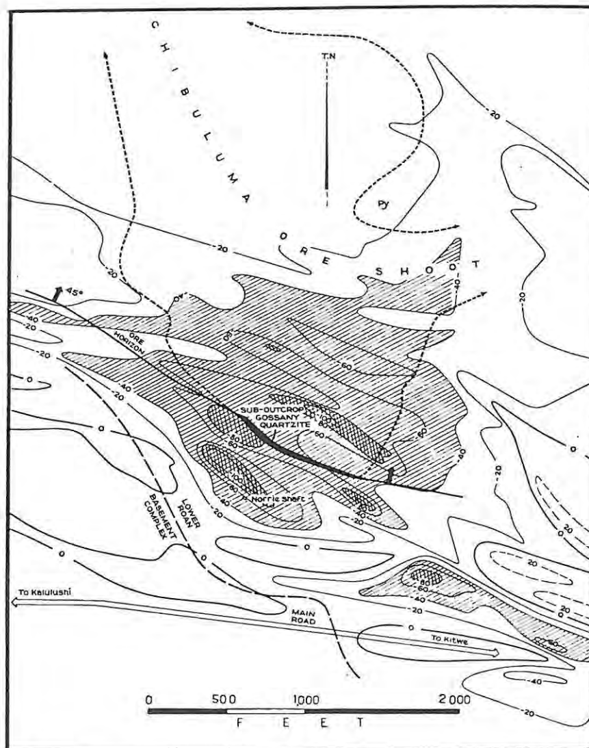
Figure 35. Chibuluma. Self-potential contours (millivolts) above Chibuluma orebody. The minus 60 millivolt contour coincides with the plan projection of the shallower part of the ore shoot; "parasitic" anomalies occur in the footwall of the orebody (from Mendelsohn, 1961).
