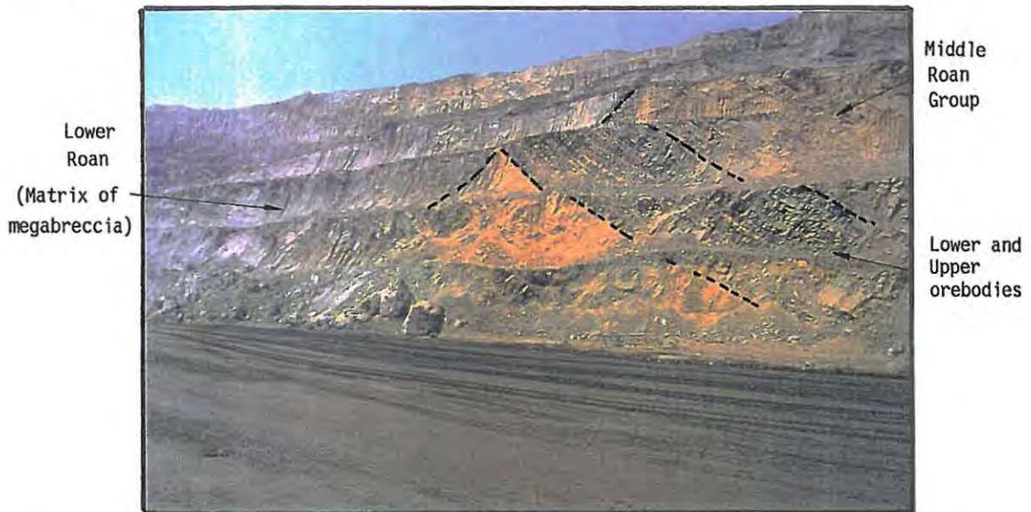
Photo 2. KOV open-pit showing Middle Roan stratigraphy as well as megabreccia (from J.E. Potgieter).
