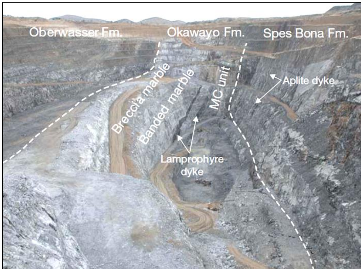
Figure 11: A schematic diagram of the Navachab open pit looking to the NNE. The lithological formations exposed include the Spes Bona, Okawayo and Oberwasser which all dip steeply towards the WNW (to the left of the diagram). Mineralization is hosted by quartz-sulphide veins crosscutting the sub-vertical lithologies. The host rocks are intruded by numerous pegmatite, aplite and lamprophyre dykes with concordant and discordant contact relationships (from Kitt, 2008).
