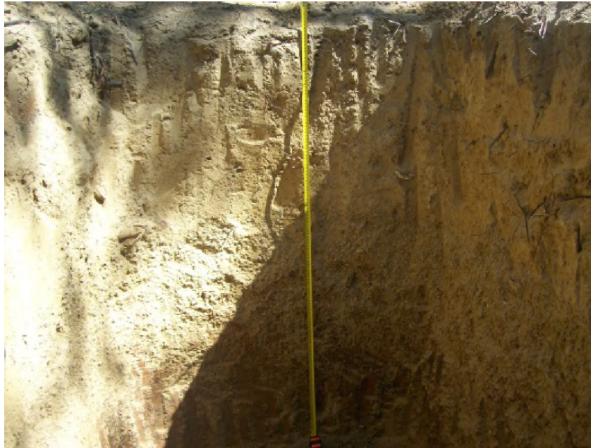
Figure 15: Orientation pit used to check optimal soil horizon for sampling.
