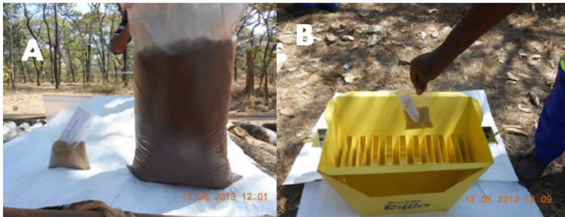
Figure 16: Sample size collected in the field. (A); average bulk sample with smallest sieved sample size; (B); smallest sieved fraction could not be spilt by Riffler without bias.
