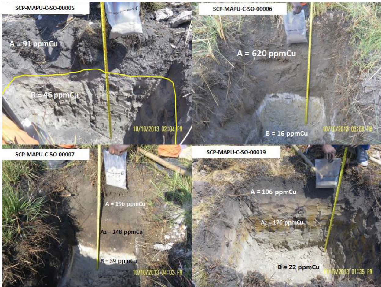
Figure 56: Sample pits dug in dambo to ascertain source of anomalous copper. In all the pits copper concentration decreased from the surface downwards.
