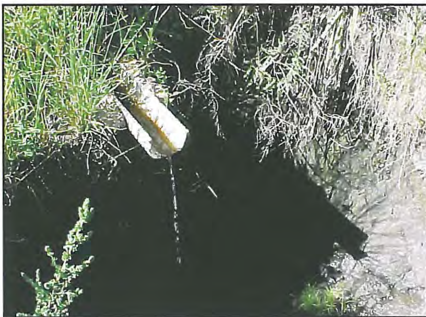
Plate 4.3: A gutter used as a discharge measuring instrument at the bottom end of the seep wetland where it joins the main wetland.
