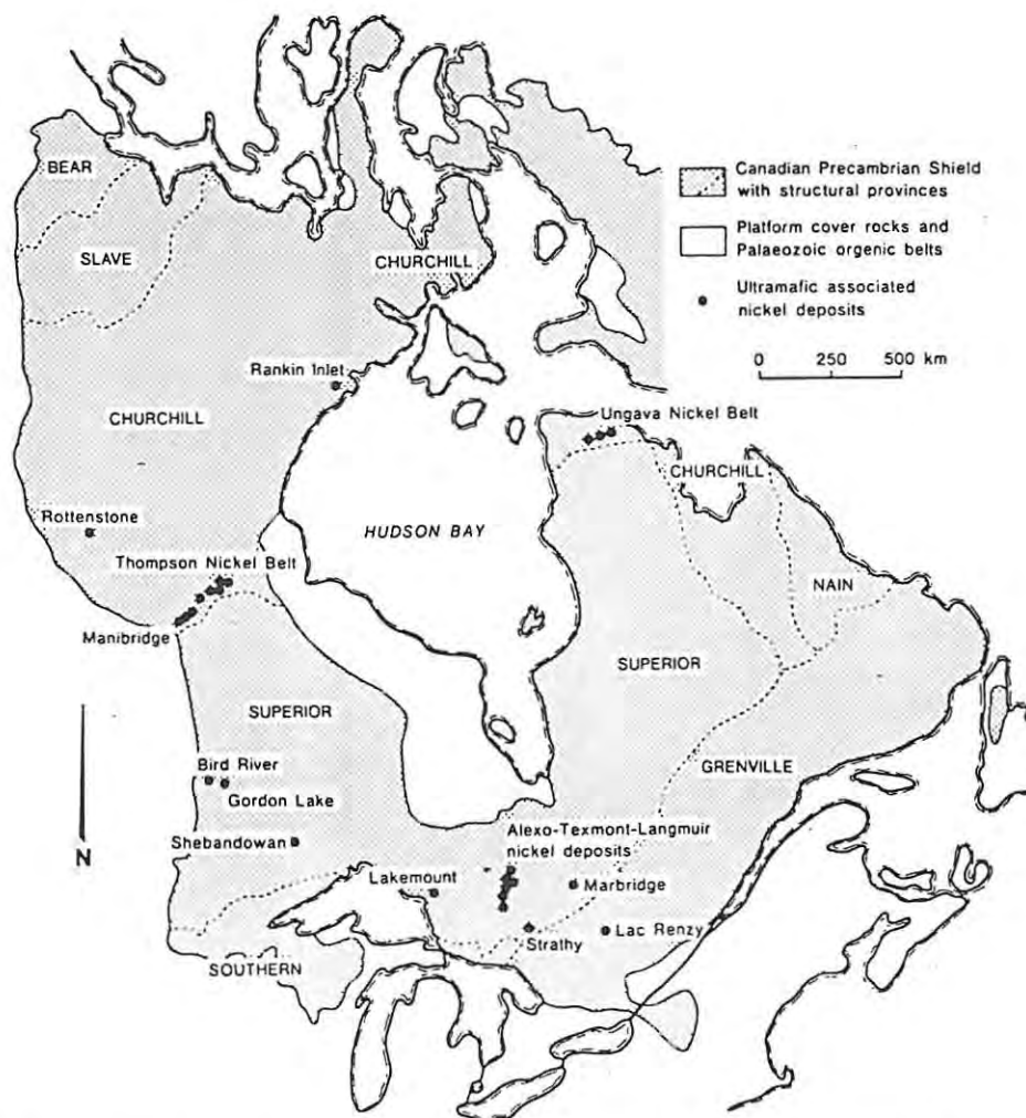
Fig. 5.3. Location of ultramafic-associated nickel deposits in Canada in relation to major structural provinces of the Canadian Shield (after Kilburn et al., 1969; from Groves and Hudson, 1981).
