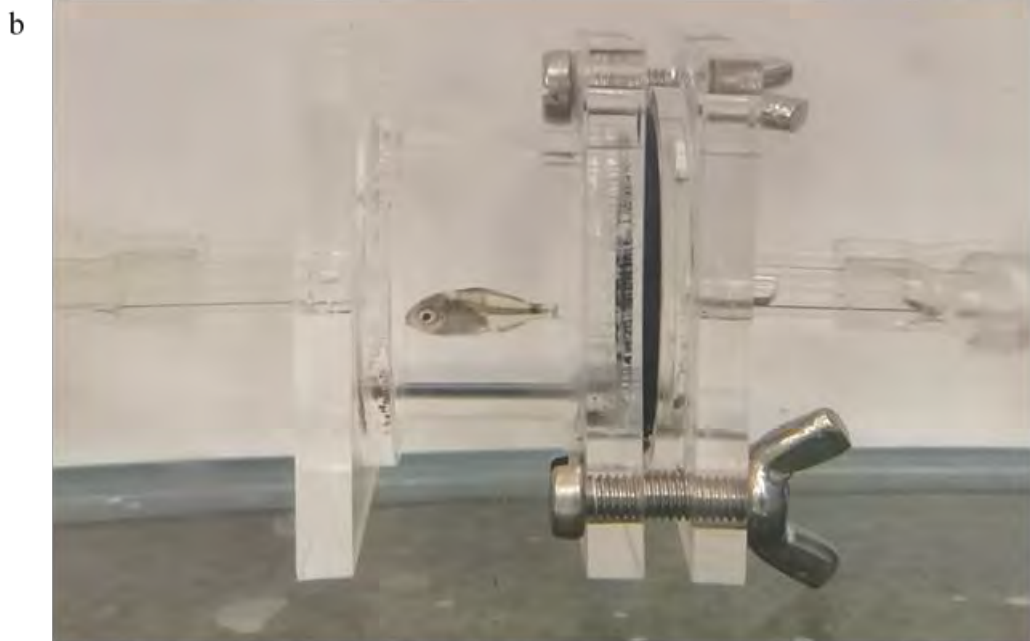
Figure 4.1: a) Schematic diagram of the respirometry system showing the flow circulation within one of the four respirometry chambers used for each trial and b) image of a post-flexion stage Diplodus capensis housed in a custom made flow through respirometry chamber
