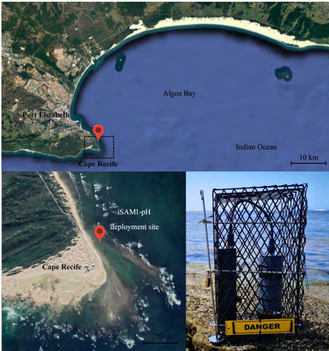
Figure 3.1: Map of the location of the iSAMI-pH deployment site at Cape Recife ( 34^{\circ}01'36.9''\text{S} 25^{\circ}42'03.2''\text{E} ) and image of the iSAMI-pH logger housed in the stainless-steel cage
