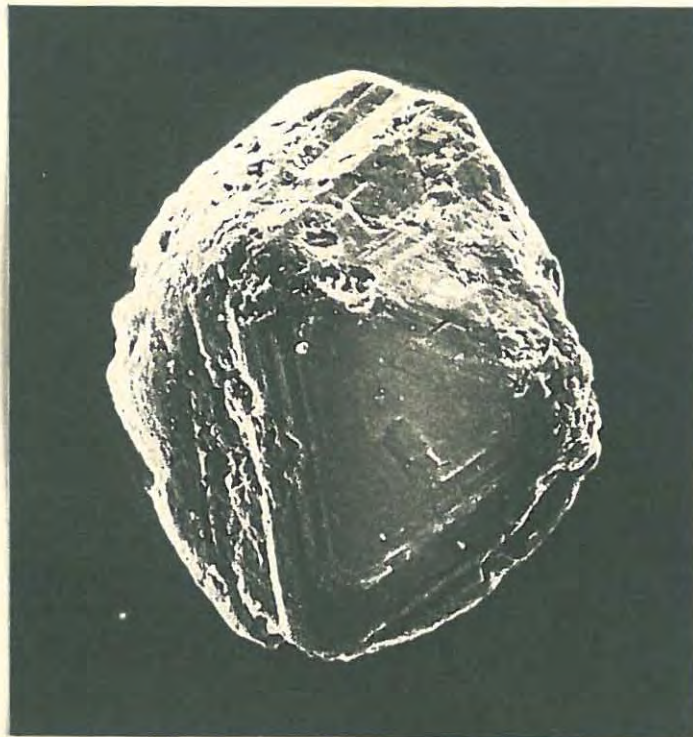
Fig. 28 SEM micrograph of detrital titanomagnetite grain, notice euhedral shape and pitted surfaces (magnification: 1 000 x).
