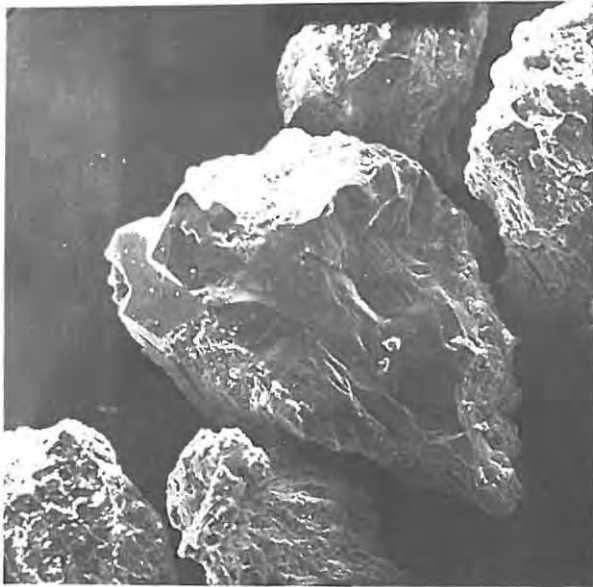
32 a Secondary silica overgrowth, notice pyramidal faces of new quartz growth (Magnification 300 x).
