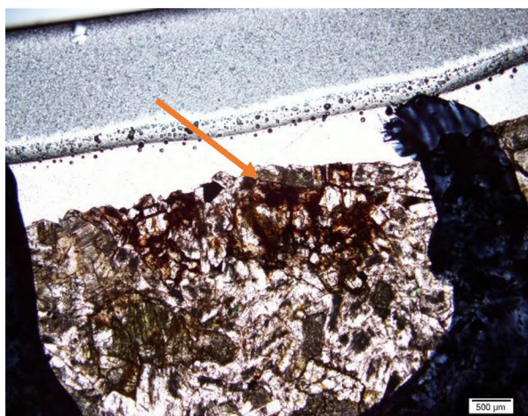
Figure 7.6.1: Opacity changes (clear to reddish-brown) at the external surface of Robertskollen (Knox 3). Arrow indicated the zonation of the discolouration
