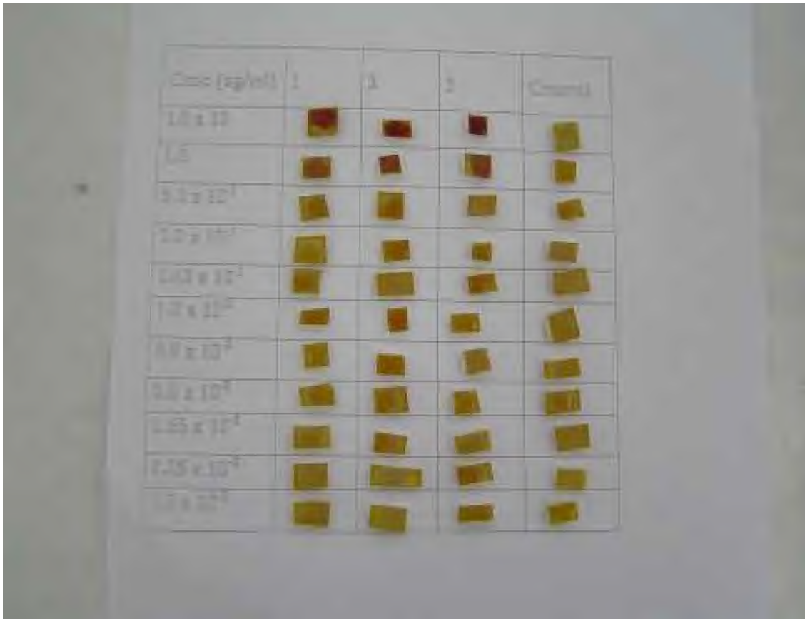
Figure 6.4: Colour changes due to immobilised CPRG hydrolysis by different commercial B-GAL concentrations.
