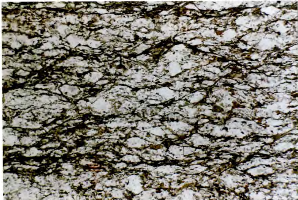
Fig. 17: Photomicrograph (uncrossed polars) of the basal quartz-biotite schist. Field of view is 4 mm.
