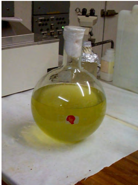
Figure 4.5 Photograph of reactor effluent collected on days 12-15 of the investigation. The green-yellow colour is indicative of the presence of polysulphides.
