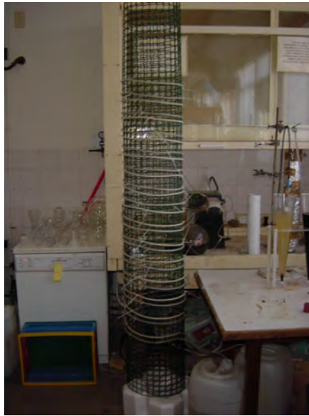
Figure 6.2 Photograph of the Silicone Tubular Reactor laboratory set-up. Silicone tubing was supported on a plastic mesh column
