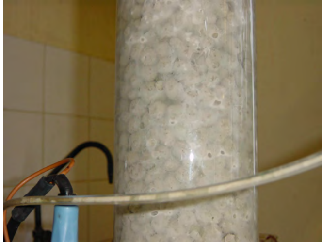
Figure 5.11: Photograph of drowned trickle filter reactor showing white sulphur accumulation on the reactor walls
