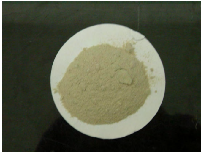
Figure 6.6: Photograph of dried biofilm harvested from Silicone Tubular Reactor.
