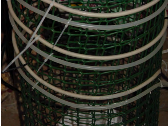
Figure 6.5: Photograph of silicone tube reactor showing white biofilm development within the tubing (top tube) compared to a fresh length of silicone tubing.
