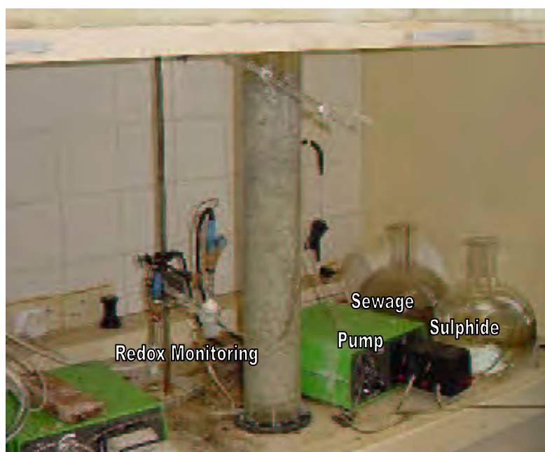
Figure 5.2: Photograph of laboratory set-up of drowned trickle filter
