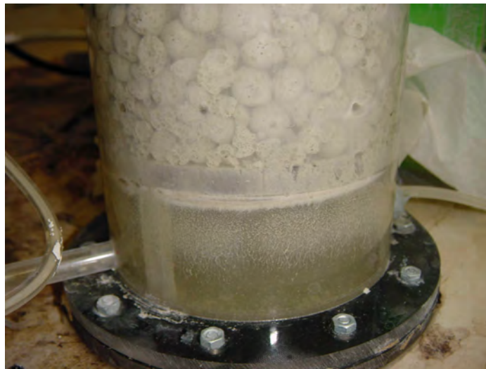
Figure 5.12 Photograph of drowned trickle filter reactor showing white sulphur accumulation and filamentous bacterial growth on the reactor wall
