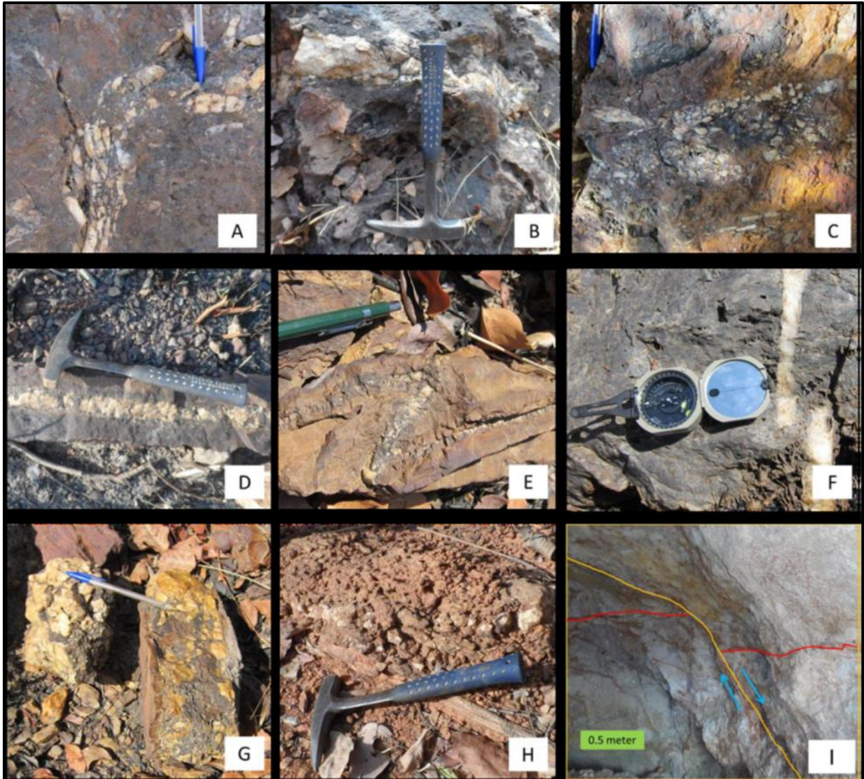
Figure 49: (A) & (E) Folded veins, varying from tight to open, from ar. (B) Highly ferruginised greywacke with quartz veining. (C) Ferruginised greywacke and siltstone units play host to a 10cm thick quartz vein. (D) Quartz vein scree material at area 1, similar sized scree boulders were observed across the target. (F) An interpreted calcareous chert or a calc-silicate unit outcrops at area 4. (G) 15cm thick quartz vein scree found. (H) Quartz vein in saprolite mined. (I) interpreted normal fault highlighted by the orange line as it displaces a quartz vein (red).
