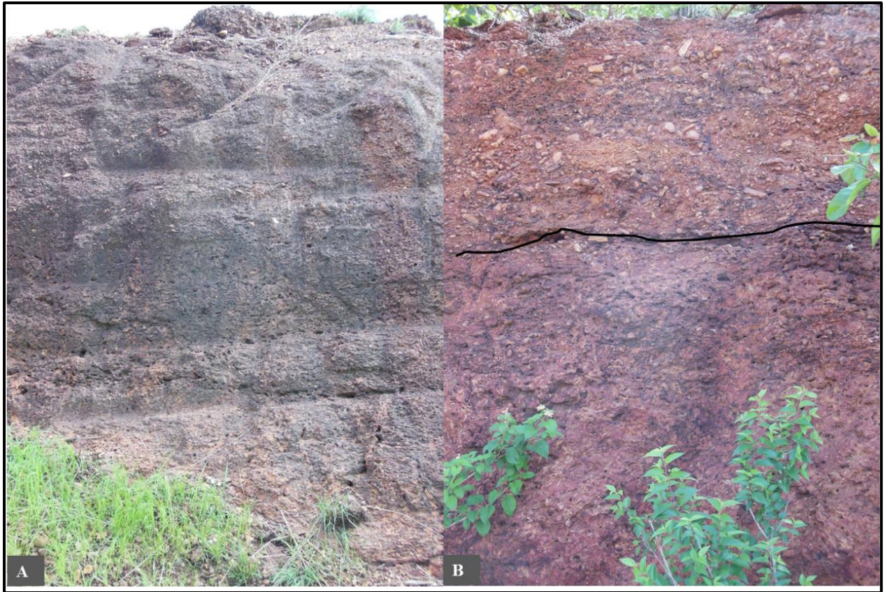
Figure 20: Photographs ‘A’ and ‘B’ showing typical exposures seen in outcrop (December 2013). ‘A’ is a strongly indurated ferruginous duricrust developed in transported material. A coarse-grained, clasts-rich upper colluvium grades downwards into a less indurated, finer matrix with sparser clasts. Alluvium at the base of the section is indurated predominantly by silica rather than iron oxides. ‘B’ photograph shows a cuirasse with polymictic clasts.
