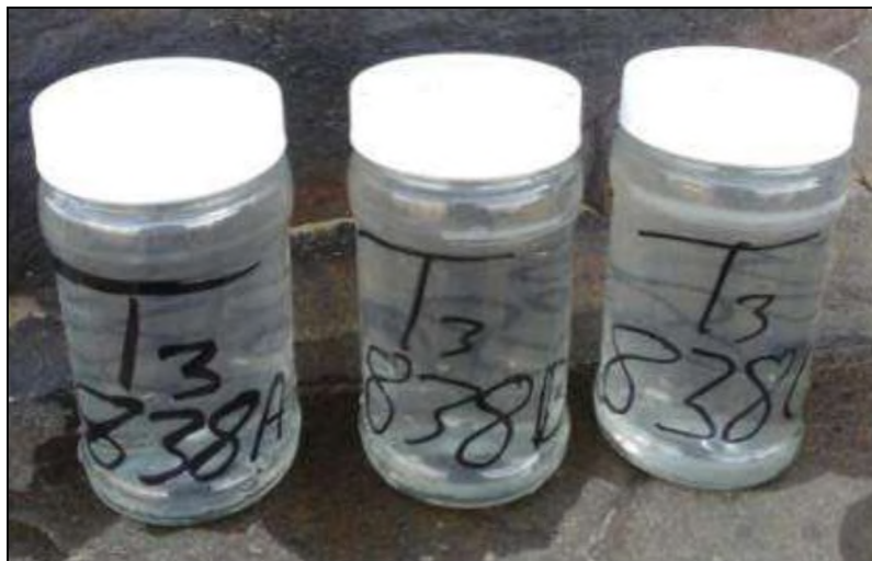
Plate 6: Sample photograph from an ODK record showing a “triple” sample, denoted by the same sample number plus ‘a’, ‘b’, ‘c’
