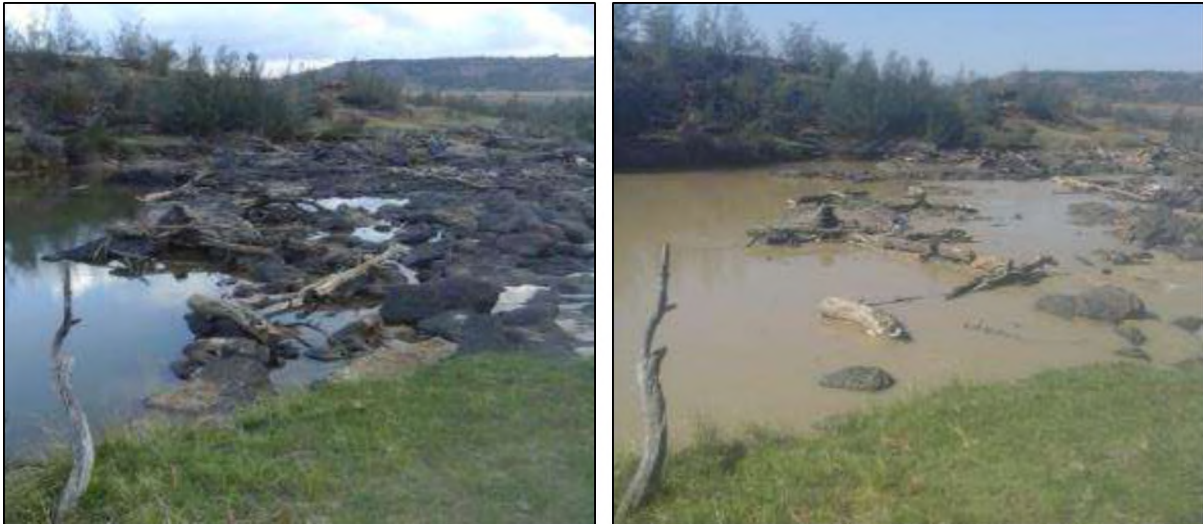
Plate 10: Photographs of the Tsitsa River at The Falls from ODK forms, showing the use of “telltales” to determine low and high water depth at the monitoring site
