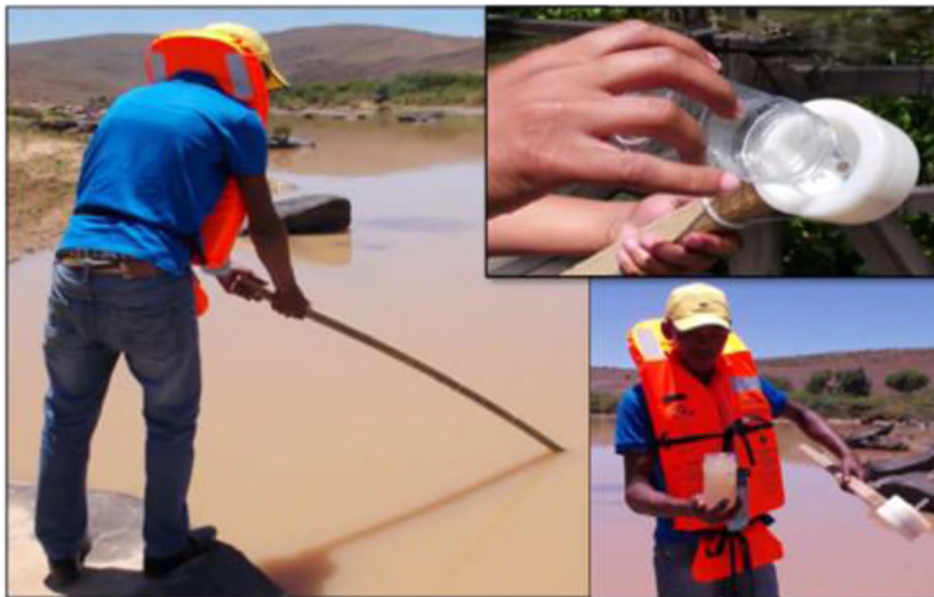
Plate 7: The wooden pole sampler in use showing the head assembly and sample jar (Bannatyne et al. 2017)
