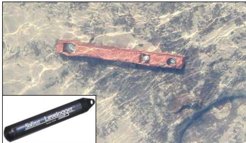
Plate 9: A pressure transducer (inset) in its steel housing attached to bedrock at a monitoring site in the Tsitsa River catchment
