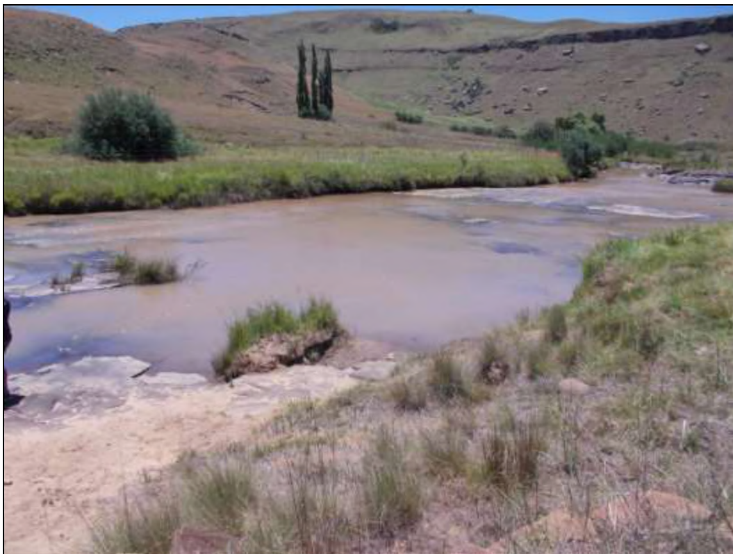
Plate 5: The flow-gauging site on the Pot River at Vipan, showing the stable bedrock channel: the sampling site closer to the CT's home has no suitable outcrop for attachment of the pressure transducer
