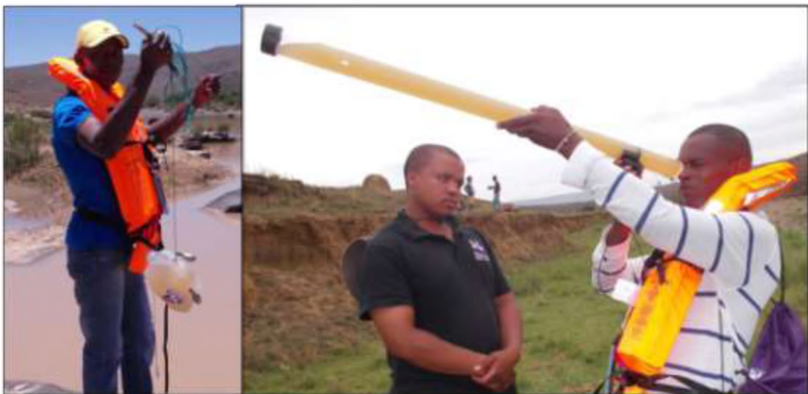
Plate 8: Visual clarity estimation using a weighted milk-bottle and GroundTruth clarity tube
