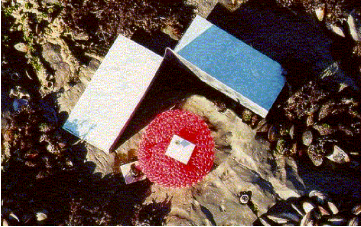
Plate 3.1: Nylon pot scouring pads were used for the collection of Perna perna larvae. Half of the pads had L-shaped metal baffles attached around them as shown. The pads were individually numbered with aluminium tags attached to the substratum.
