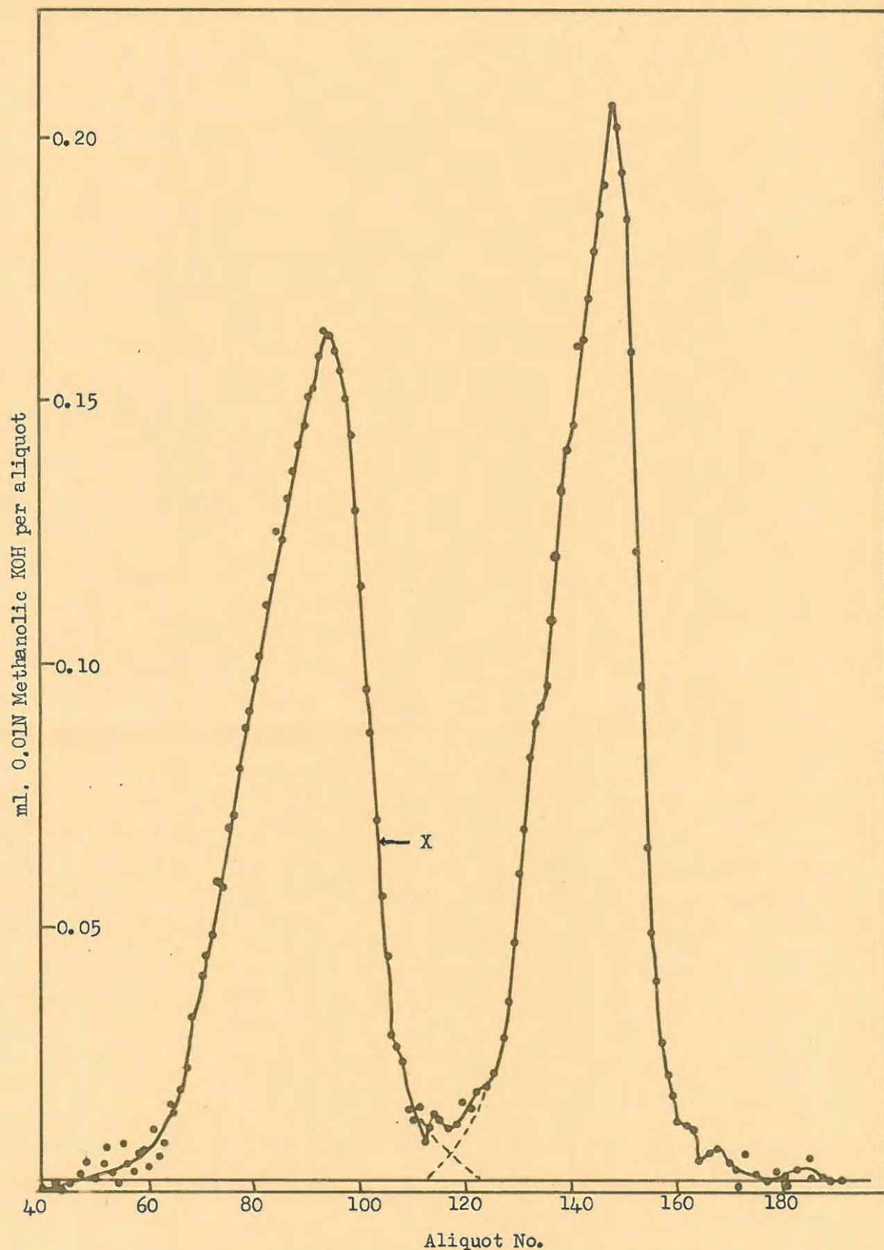
Fig. IV. Chromatographic Resolution of a Mixture of Oleic ( C_{18} monoene) and Linoleic ( C_{18} diene) Acids.
