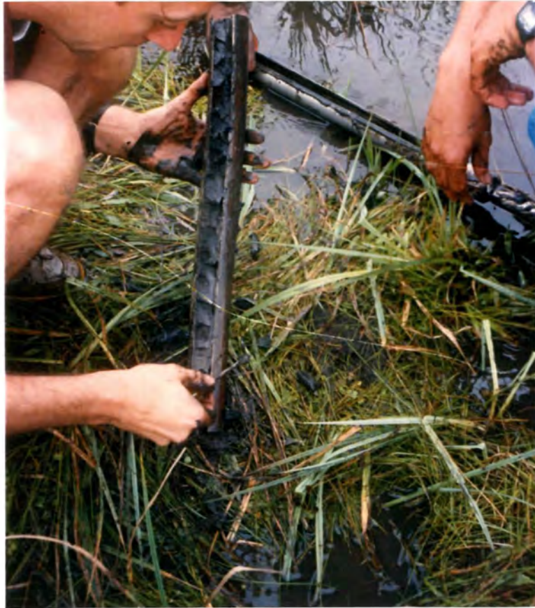
Plate 31. Hiller borer — restricted sampling depth.
