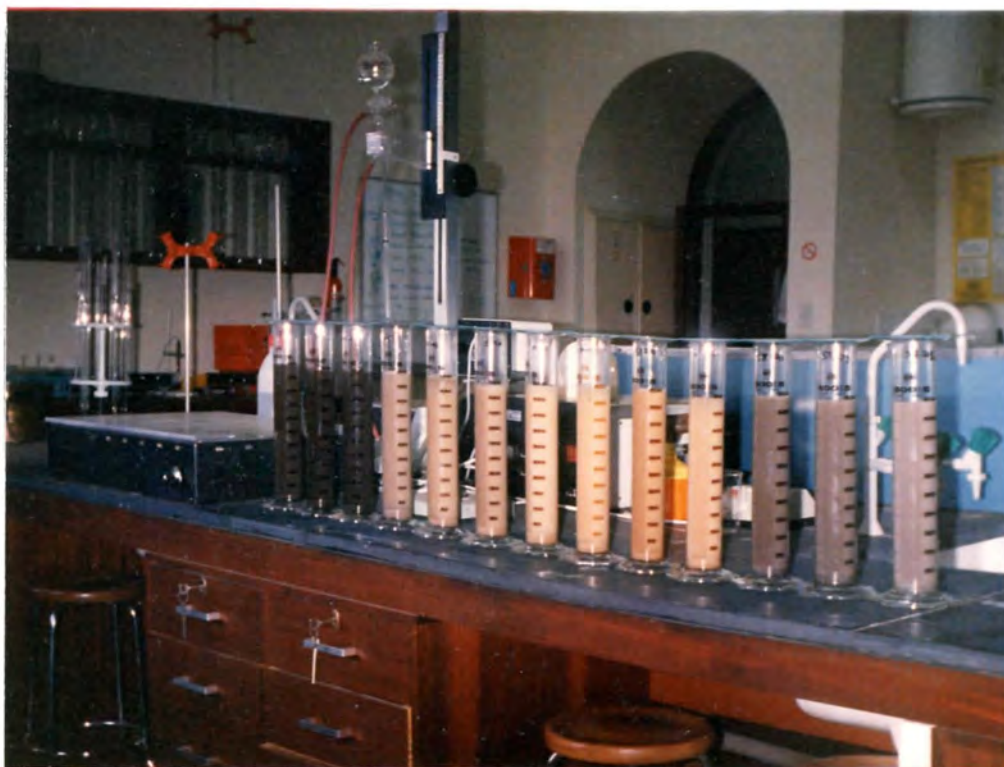
Plate 39. Sedimentation cylinders of dispersed sediment. Scale 1:13
