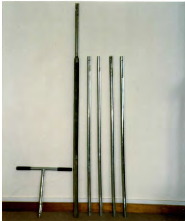
Plate 32. Gouge auger and extension rods. Scale 1:12
