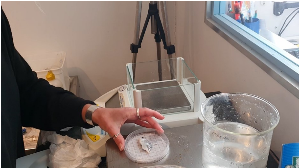
Figure 2. 6: The process of measuring and weighing each individual using a petri dish and millimetric paper glued underneath.
