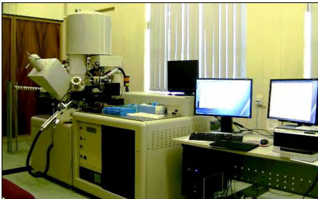
Figure A5.1: The equipment setup of the Kratos Axis Ultra DLD XPS used in this study.
