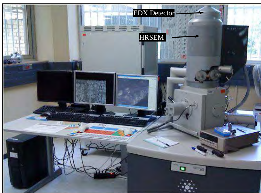
Figure A2.1: The equipment setup of the FEI Nova 230 high resolution scanning electron microscope (HRSEM) with an EDAX X-ray microanalysis module for energy dispersive microanalysis (EDX) measurements used in this study. Image courtesy of Dr. R.D. Brimecombe.
