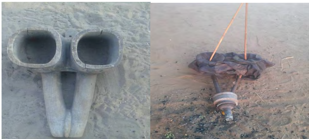
Figure 5.2: Shows the original traditional blast furnace (left)
