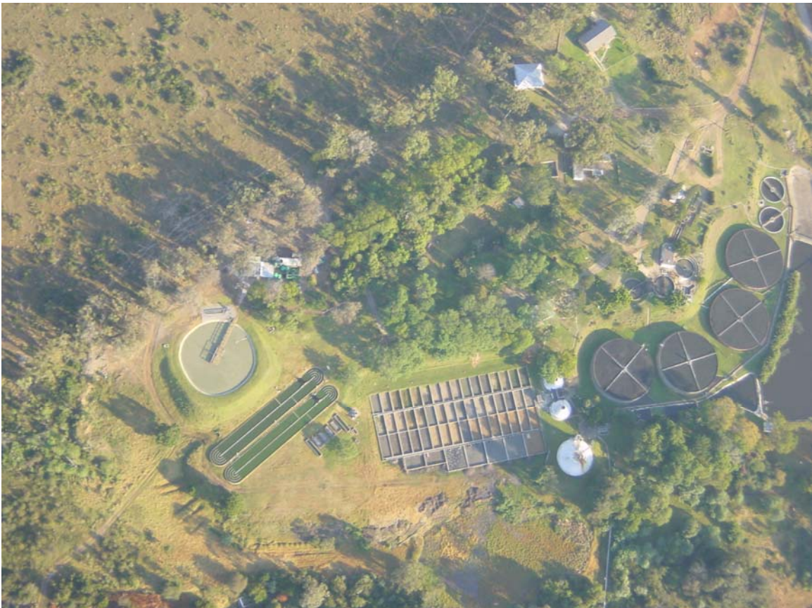
Figure 2.6: The integrated algal ponding system at left, in relation to the Grahamstown Disposal Works at right.
