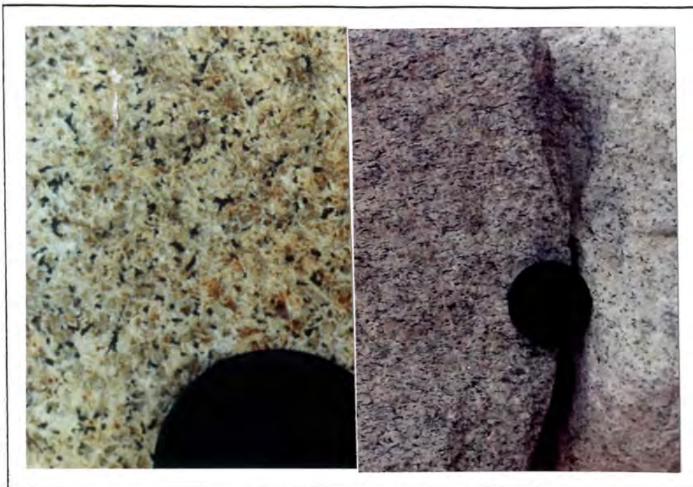
Plate 3.5 Textural variation of foyaitite. The plate on the left shows the more common intergranular, or 'foyaitic', texture produced where nepheline (now partly altered and red-brown in colour) lies in a network of tabular perthite grains. The plate on the right shows a foyaitite with a foliation produced by alignment of perthite (and hence also of interstitial amphibole).
