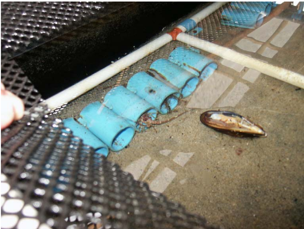
Figure 2.4: The PVC hides consisted of 25 mm piping cut to 100 mm lengths. Each tank was provided with 27 pipes.
