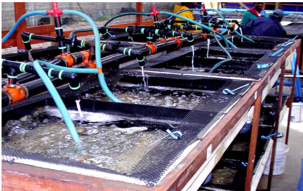
Figure 2.1: The experimental system consisted of fibreglass tanks painted black with epoxy paint. Each tank had separate water inflow and drainage with oyster mesh fitted along the top edge to prevent lobsters from escaping.
