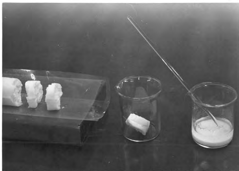
Plate D Division of the cellulose column into sections before locating the sugar bands
