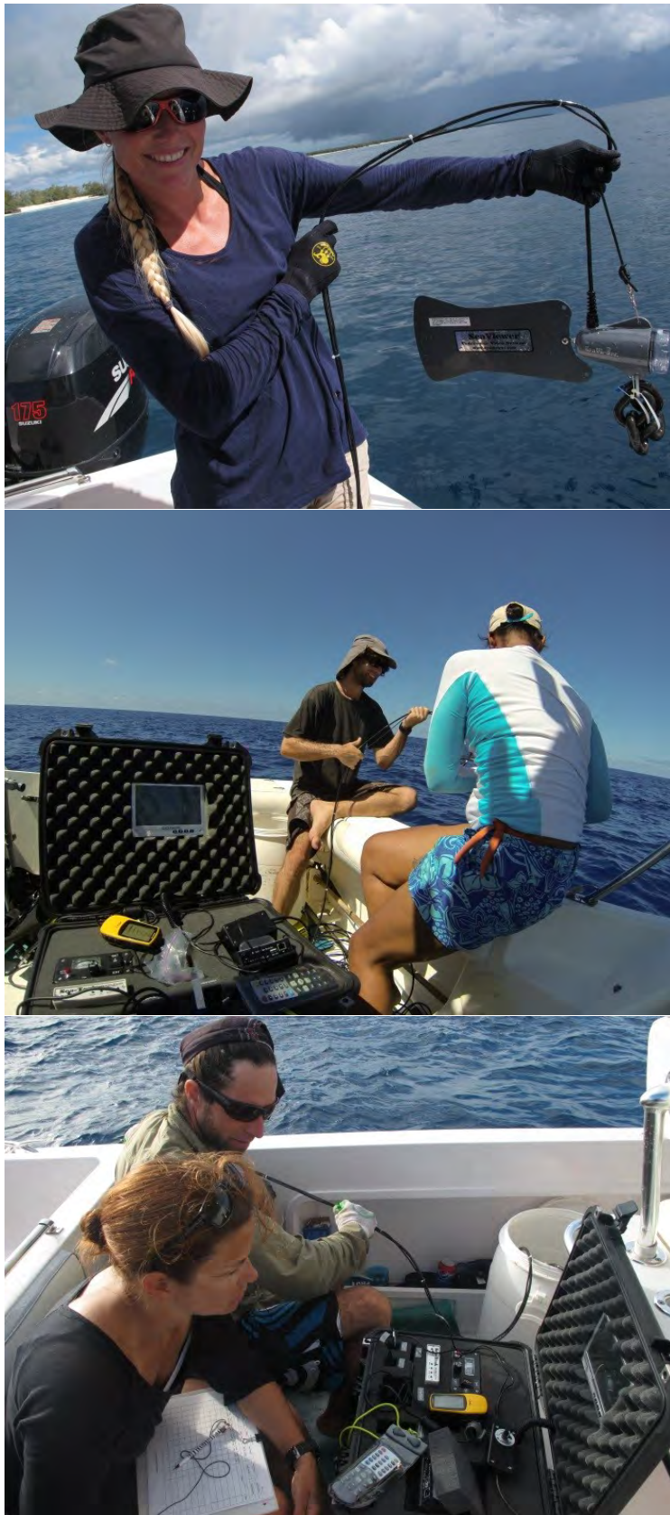
Figure 2.9. SeaViewer DropCam in action a) the camera with chain links as weight and directional fin, b) the boat-based consul unit with GPS and screen, c) data recording and underwater camera piloting
