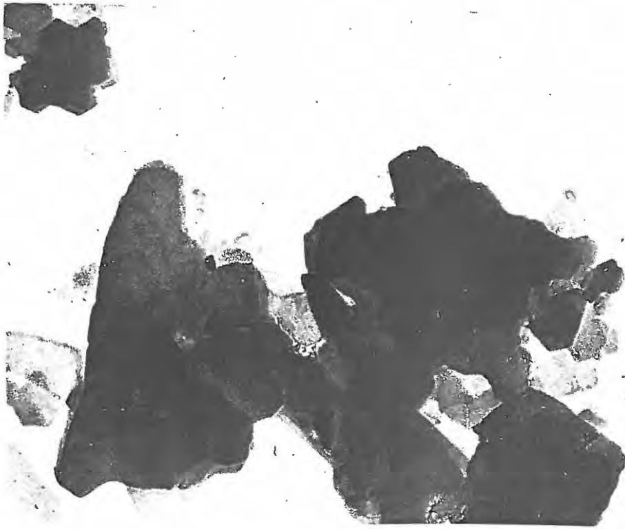
Plate 5.5 An electron micrograph of the Stowon clay. Note the aggregates of hexagonal crystals of kaolinite.
