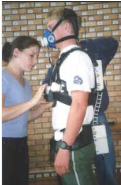
Figure 8: Subject preparation with the K4b 2 and Lumbar Motion Monitor.
