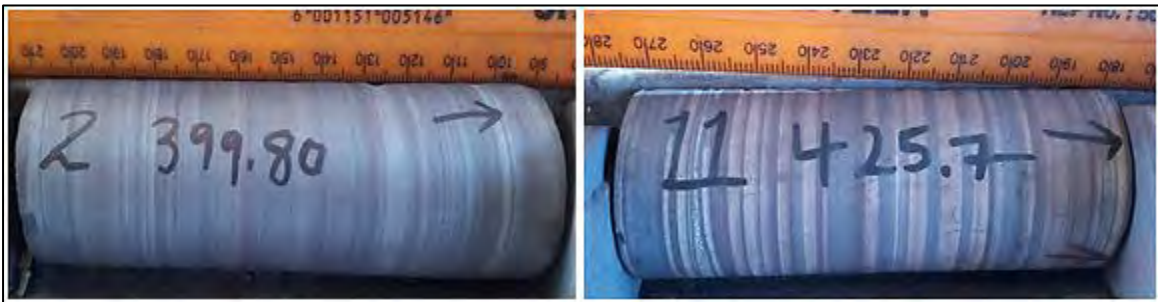
Figure 3. 2. Image of chert-hematite BIFs from borehole N95E. Depths of sampling is shown.
