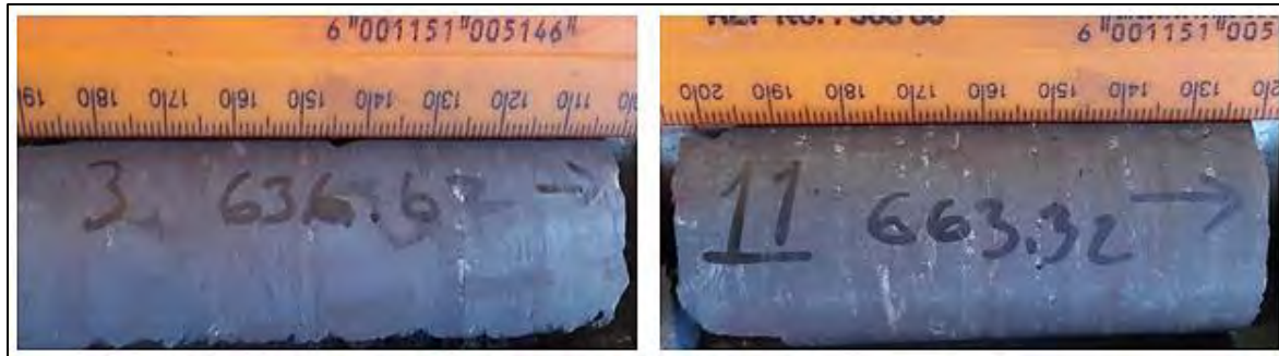
Figure 3. 9. Image of samples from the upper (left) and lower (right) Mn ore bodies of N92I.
