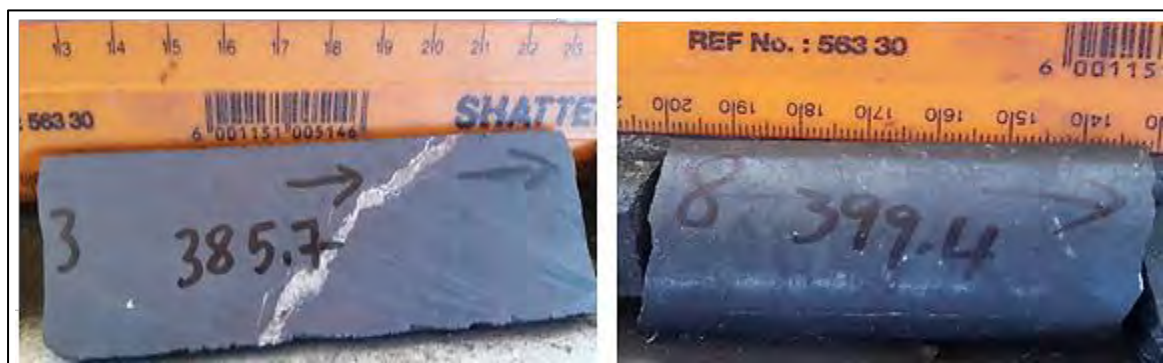
Figure 3. 5. Image of samples from the upper (left) and lower (right) Mn ore bodies of N95E. Depths of sampling are shown.
