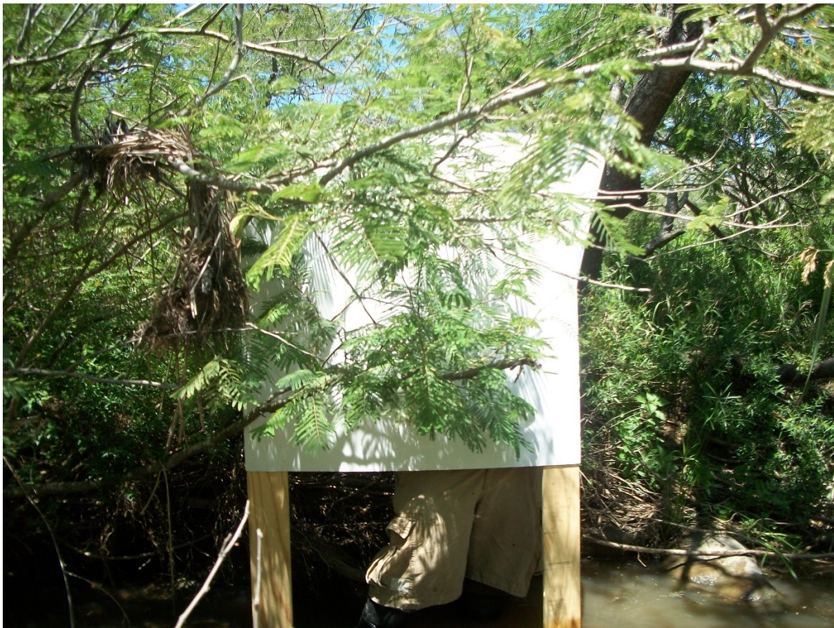
Figure 2-5: A 1 m x 1 m white board raised to 80 cm from the water surface. The board was placed behind the vegetation to estimate plant density (photo taken in February 2013).
