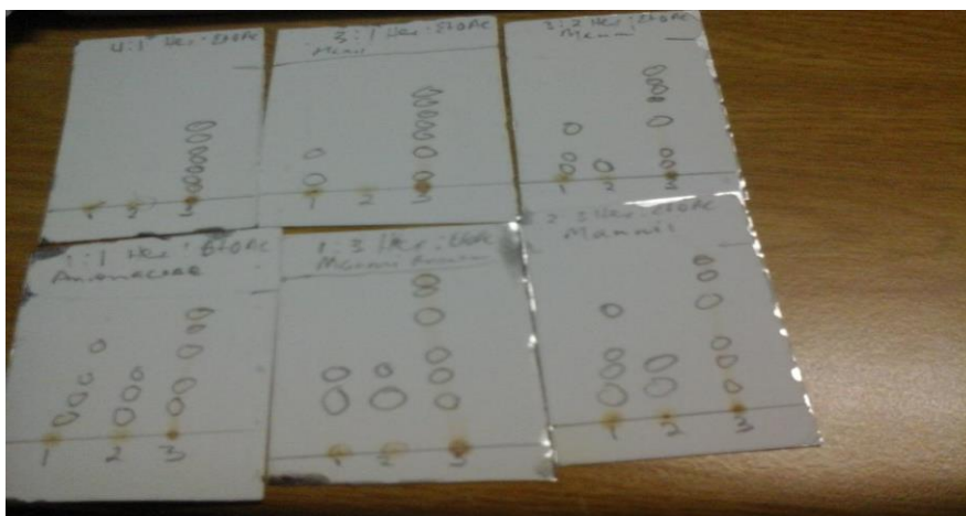
Figure 3.2: Chromatograms of crude extract dissolved in three different solvents using different mobile phase polarities
