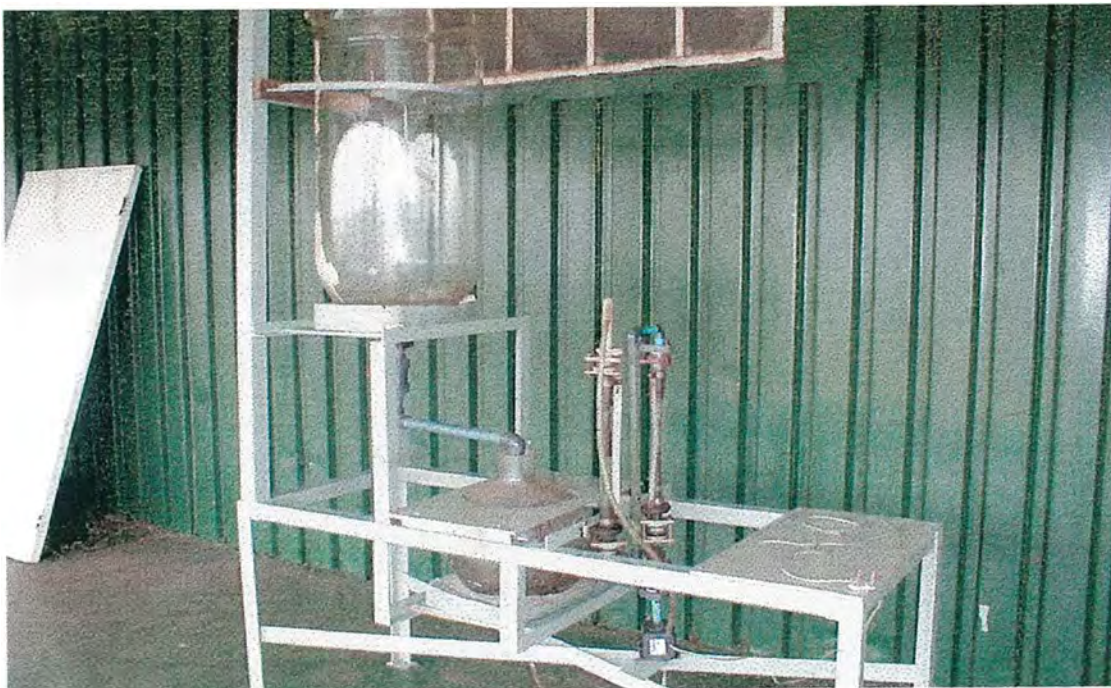
Figure 6.2 Double column construction utilised for Runs 3 to 7.
